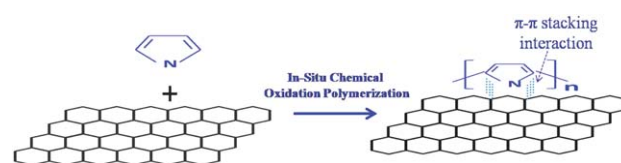
Scheme 1 In situ chemical oxidation polymerization mechanism of polypyrrole on graphene.
