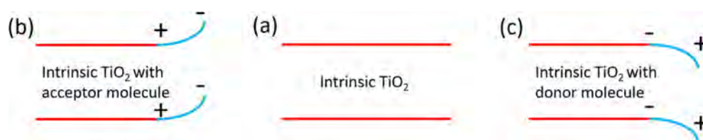
Scheme 1. Schematics of the band structure of (a) intrinsic \text{TiO}_2 , (b) intrinsic \text{TiO}_2 with an acceptor molecule, and (c) intrinsic \text{TiO}_2 with a donor molecule.
