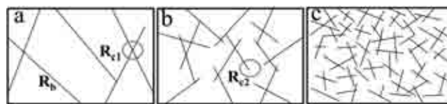
Figure 5. Illustration of thermally conductive paths for composites filled with (a) long CuNWs, (b) AgNWs, and (c) short CuNWs.
