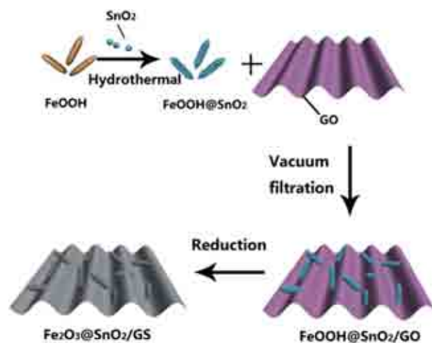
Scheme 1 Schematic illustration of the synthesis process of the Fe 2 O 3 @SnO 2 /GS film.
