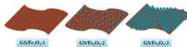
Scheme 2 A schematic illustration of the GS/Fe 3 O 4 composites with different Fe 3 O 4 content.
